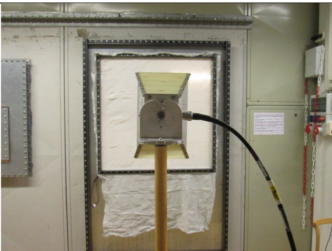
Test setup: 1 GHz – 18 GHz, horizontal, TX
