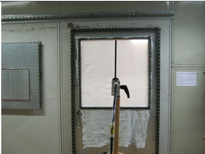
Test setup: 270 MHz – 1000 MHz, vertical, TX
