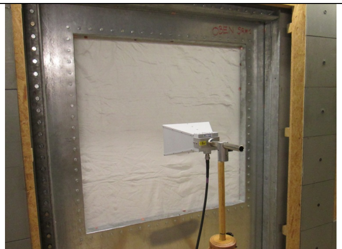
Test setup: 1 GHz – 18 GHz, vertical, RX
