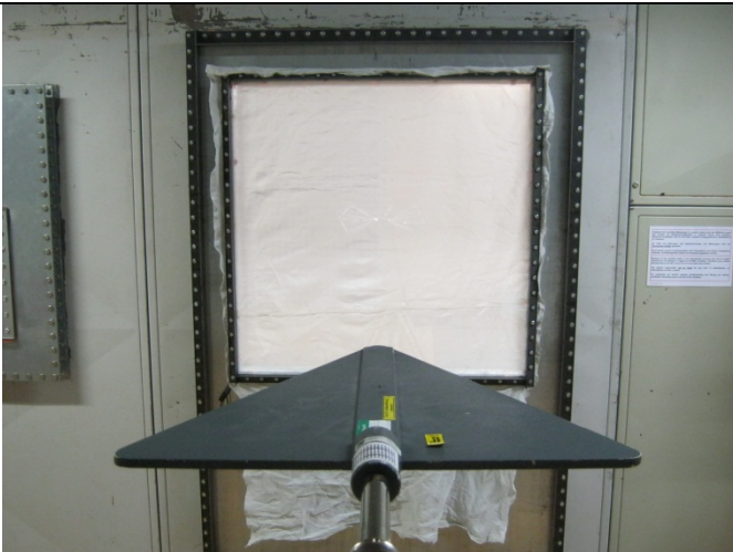
Test setup: 270 MHz – 1000 MHz, horizontal, TX
