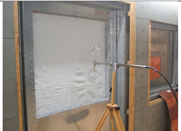
Test setup: 270 MHz – 1000 MHz, vertical, RX
