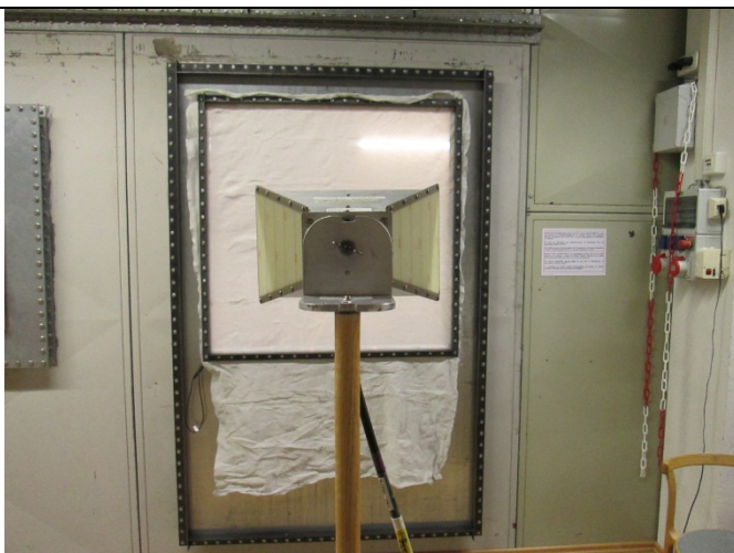
Test setup: 1 GHz – 18 GHz, vertical, TX
