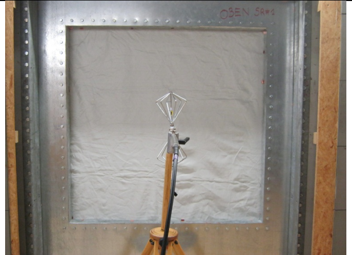
Test setup: 30 MHz – 270 MHz, vertical, RX
