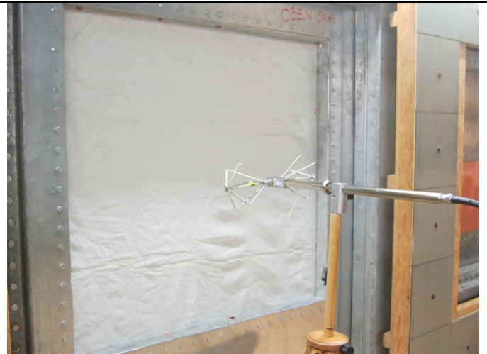
Test setup: 270 MHz – 1000 MHz, horizontal, RX
